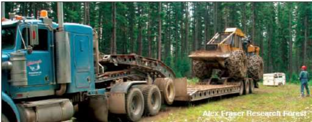
Figure 2. Check machinery prior to movement & clean as needed to prevent the spread of invasive species
