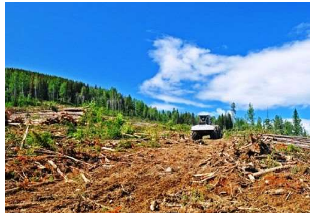
Figure 3. Proper equipment, such as this wide-tired skidder, and proper techniques to reduce the impact to soil
